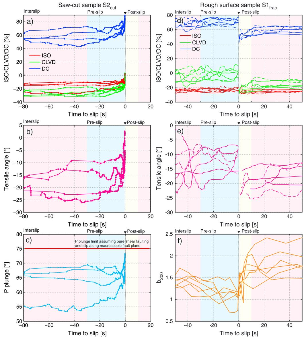
**Figure 2.** Changes in MT-derived parameters and  $b$  values before and after slip events for (a–c) experiment  $S2_{cut}$  and (d–f) experiment  $S1_{frac}$ . Time  $t = 0$  s corresponds to the slip onset and is marked with inverted triangle. Dots show places at which moving averages were calculated (Figures 2a–2c).
